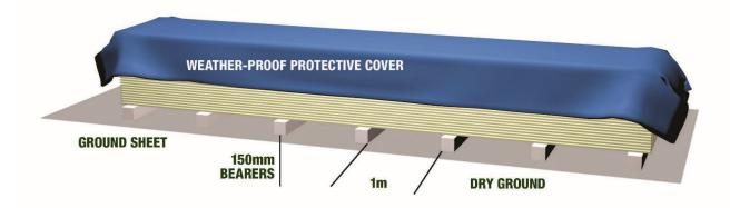
Ensure the product is stored on site correctly. Inside, under cover or as per the diagram above if stored outside.
